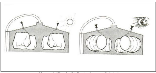
Diagram 6. "Breather Bag" system in oxygen-limited silo
