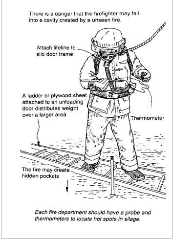
Diagram 11. Probing for hot spots in silage
