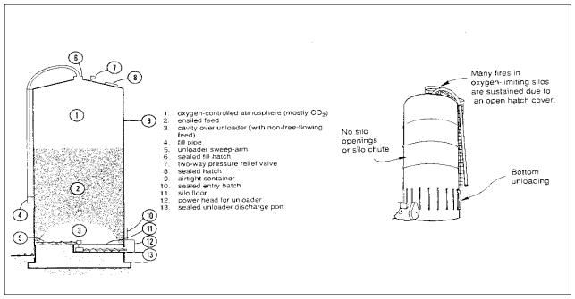
Diagrams 3 and 4. Features of an oxygen-limiting silo
