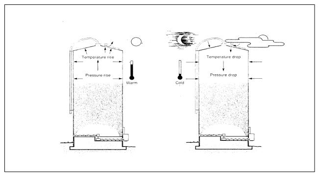
Diagram 5. Oxygen-limiting silos must "breath" to compensate for temperature and pressure changes
