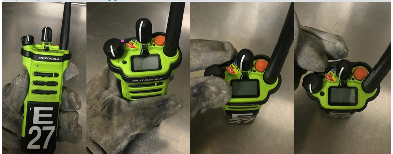
Figure 6.1. NFPA 1221 9.3.6.6: Portable radios shall be designed to allow channels to be changed while emergency response personnel are wearing gloves
