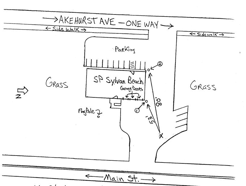
X-Starting Point - PK Surveyor's Pin 1 - Reference Point #1-Concrete Filled Steel Corner Barrier 2 - Reference Point #2-Concrete Filled Steel Corner Barrier W/ Reflective Tape W/ Reflective Tape
